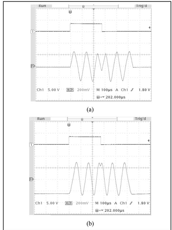
Figure 4. The measured in-phase and quadrature signals (a) I (b) Q
