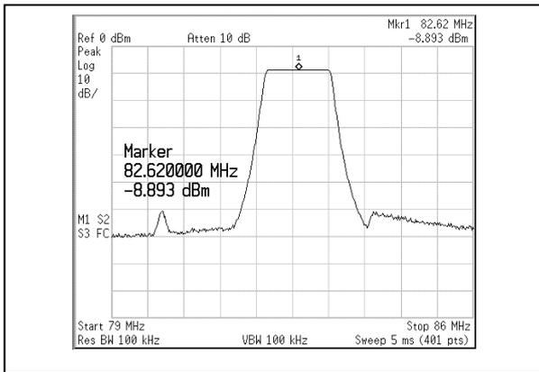
Figure 3. The spectrum of the DDS output (AD9954)
