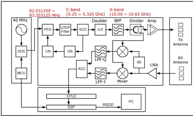
Figure 1. The block diagram of the X-band FMCW radar
