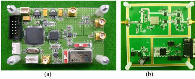
Figure 2. Baseband DDS (AD9954) and X-band PLL system
