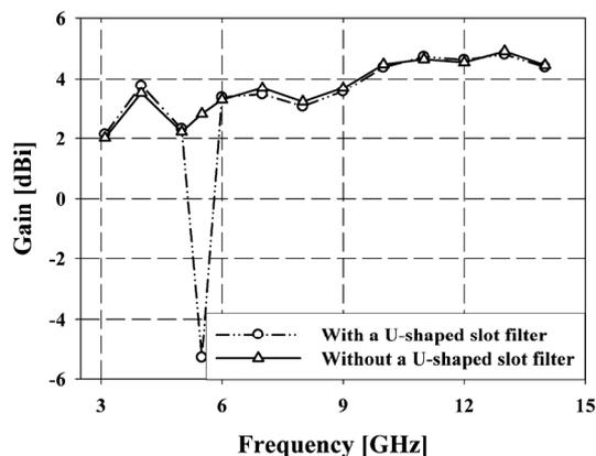
Fig. 7. Measured gains of the antennas with and without the U-shaped slot filter
