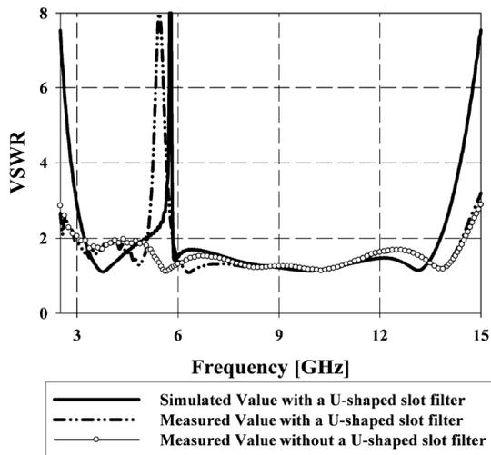
Fig. 5. Measured and simulated results of VSWR
