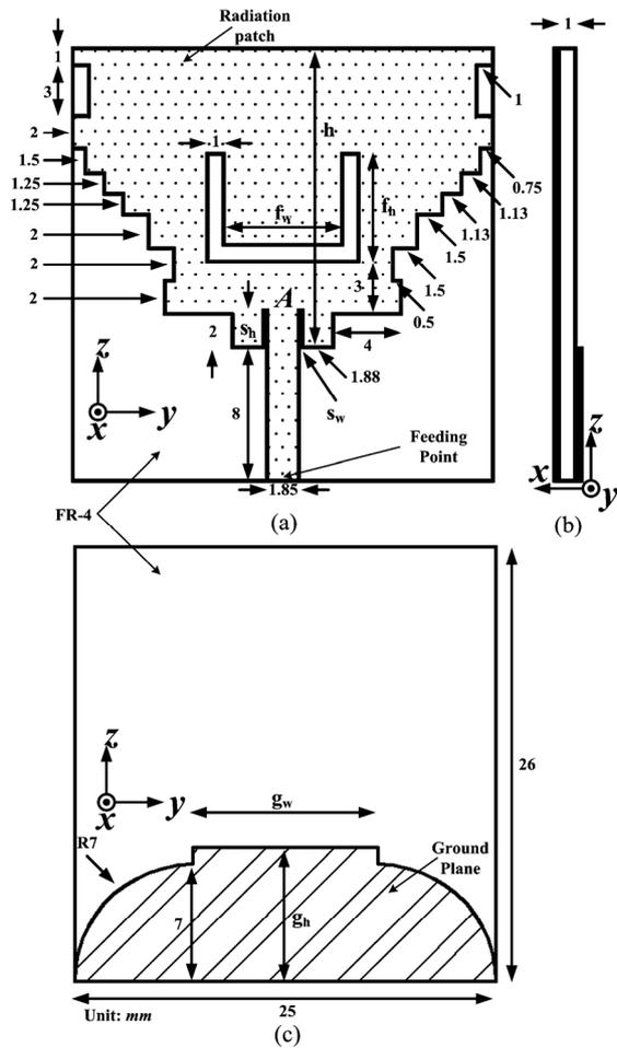
Fig. 1. Geometry of the proposed antenna
