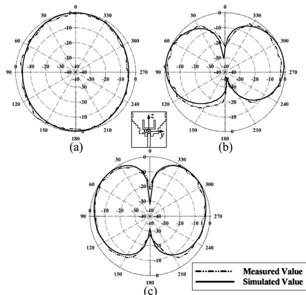
Fig. 6. Measured and simulated radiation patterns for the proposed antenna at 7 GHz.
