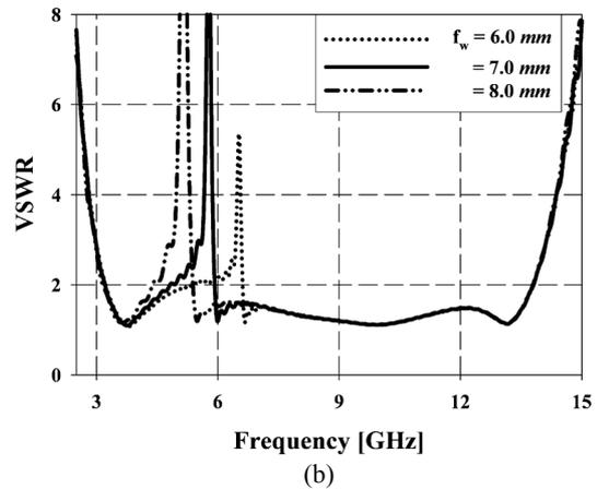
Fig. 3. Simulated VSWR as a result of the parameters of each extended ground plane
