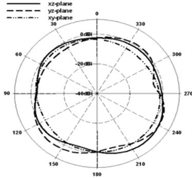
Fig.4 Calculated far filed pattern at 2.64GHz for a single PIFA in the dual element compact array.
