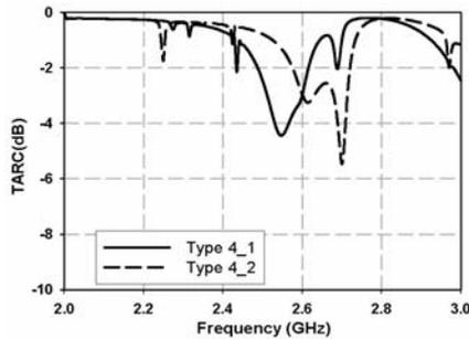
Fig. 8. TARC at 2.64GHz for four elements antenna arrays
