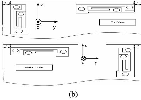
Fig.7 The proposed two types of four elements arrays. (a) Type 4\_1. (b) Type 4\_2.
