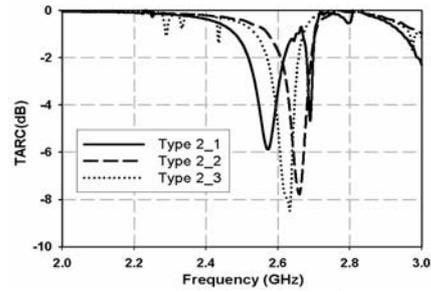
Fig.6 Calculated TARC at 2.64GHz for dual antenna arrays.
