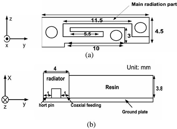
Fig.1 Geometries and dimensions of the PIFA (a) Top view. (b) Side view.
