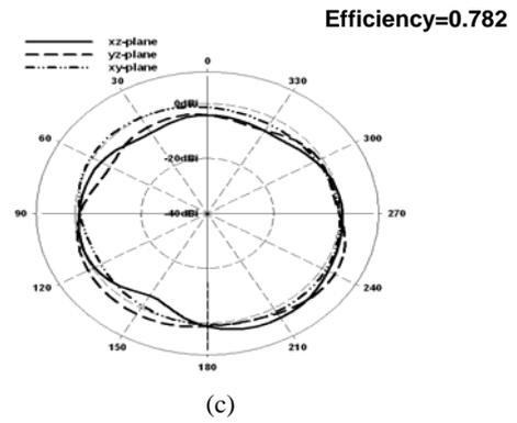
Fig.5 Calculated far filed pattern at 2.64GHz for a single PIFA in the dual element compact array (a) Type 2\_1. (b) Type 2\_2. (c) Type 2\_3.
