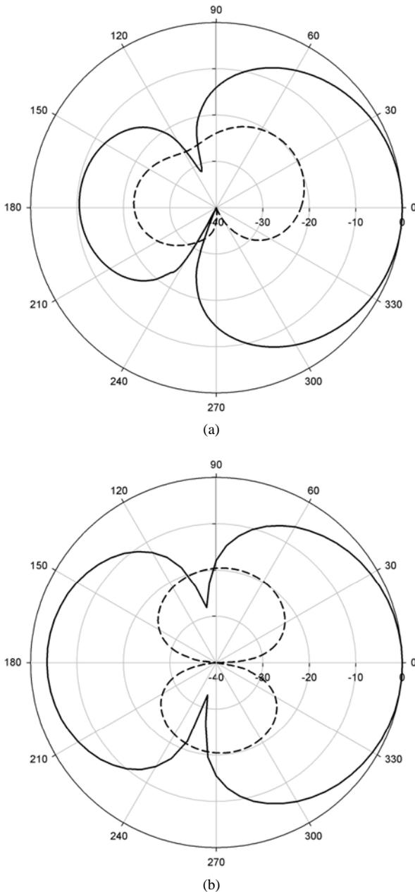
Fig. 4. (a) E-plane radiation patterns at port 1 (2 GHz). (b) E-plane radiation patterns at port 2 (2.78 GHz)
