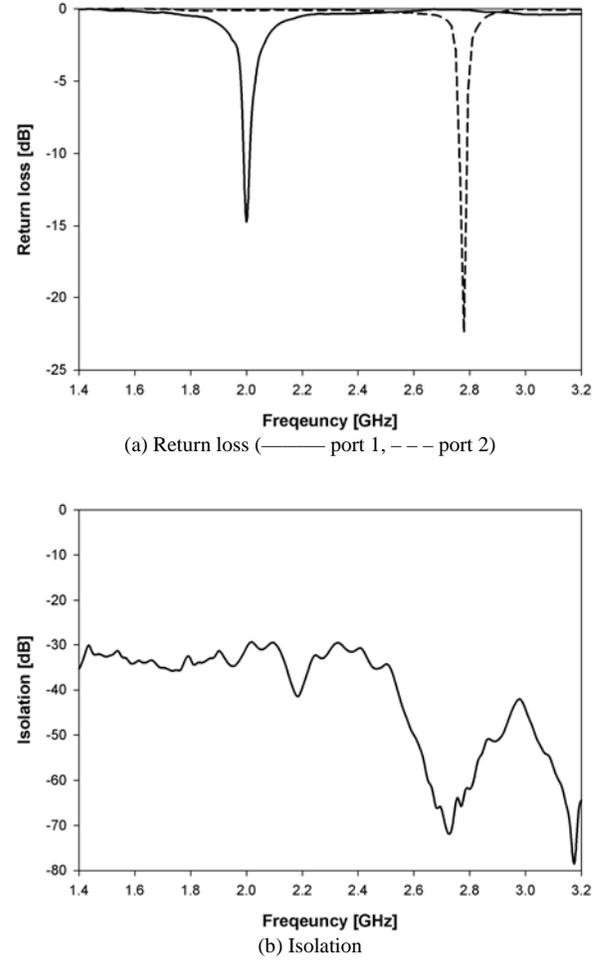
Fig. 3. Measured S-parameter for the dual-band and dual-polarization patch antenna
