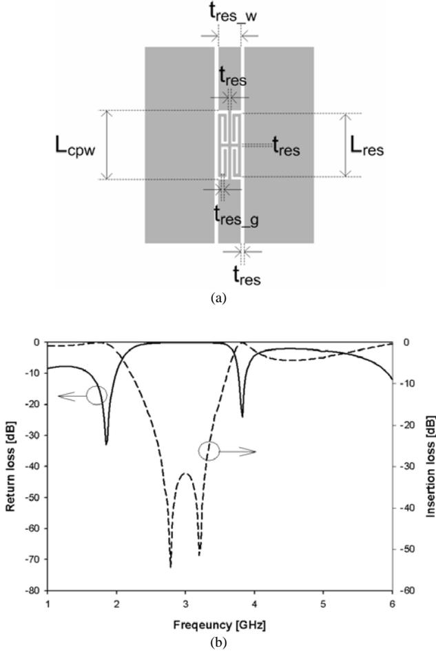
Fig. 2. (a) Configuration of the CPW resonant cell. (b) Measured S-parameters for the CPW resonant cell.
