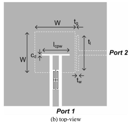
Fig. 1. Configuration of the proposed antenna.
