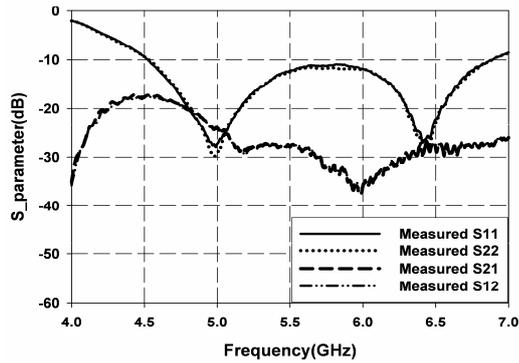
Figure 2. Measured S-parameter for the proposed antenna
