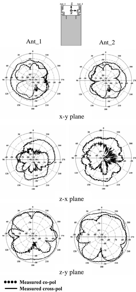
Figure 4. Measured radiation patterns at 5150MHz
