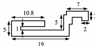
(b) Detail dimensions of the proposed antenna
