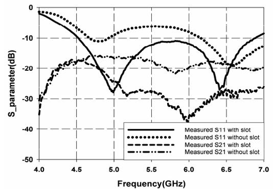
Figure 3. Measured S-parameter (with slot and without slots)
