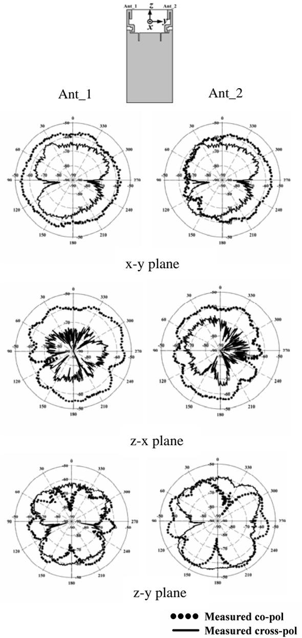
Figure 5. Measured radiation patterns at 5725MHz
