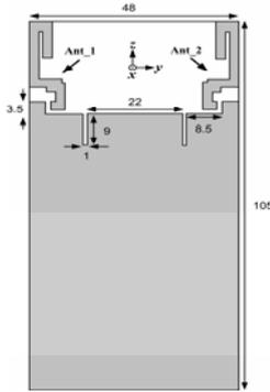
Figure 5. Geometry of the experimental model of the diversity antenna (unit : mm)
