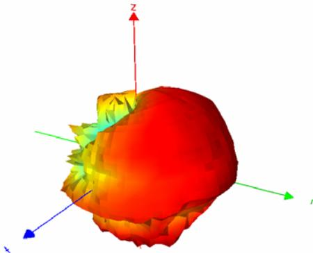
Figure 7. Measured 3D co-polarized radiation pattern of the antenna 2 of the experimental model at 5.15 GHz
