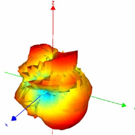
Figure 4. Measured 3D co-polarized radiation pattern of the simple handset model at 1.9 GHz
