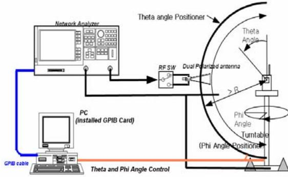
Figure 1. Spherical antenna measurement system
