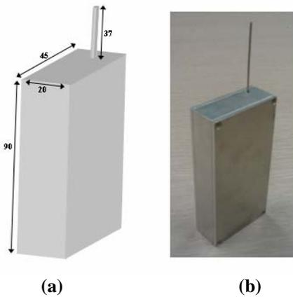
Figure 3. The monopole box (a) dimensions, (b) picture (unit : mm)
