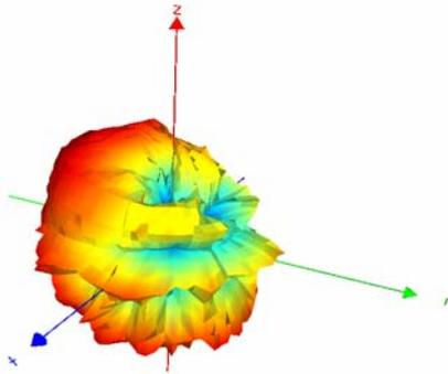
Figure 6. Measured 3D co-polarized radiation pattern of the antenna 1 of the experimental model at 5.15 GHz
