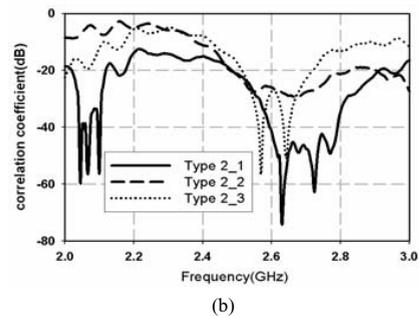
Fig.6 Calculated correlation coefficient for dual antenna array
