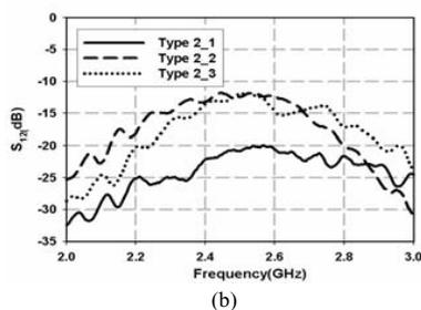
Fig.5 Mutual coupling for dual antenna array
