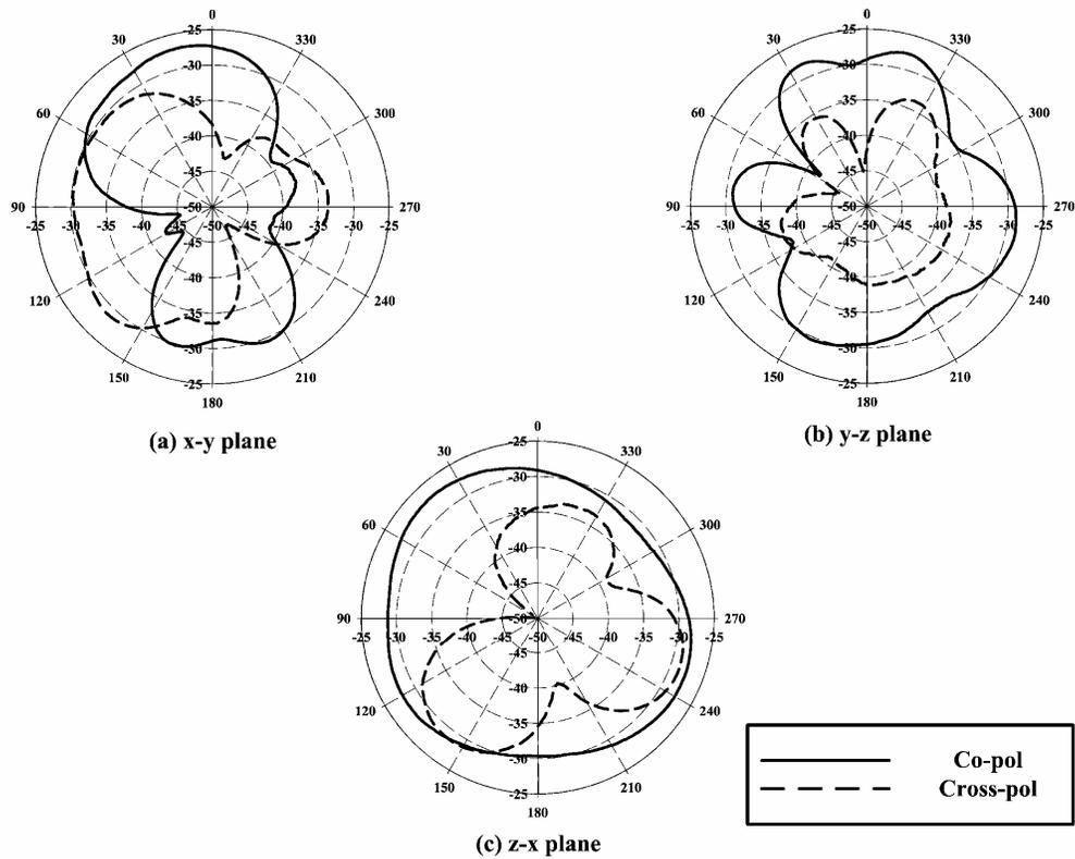
Fig. 3. Measured radiation patterns for the proposed antenna at 2.4GHz.
