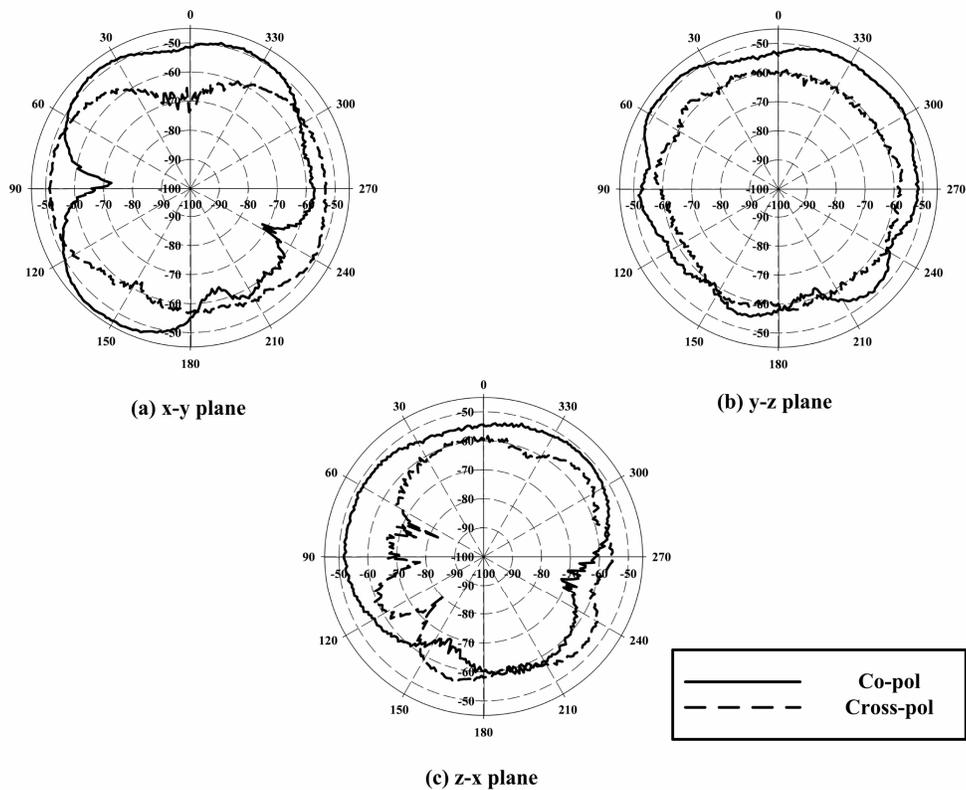
Fig. 4. Measured radiation patterns for the proposed antenna at 5.18GHz.
