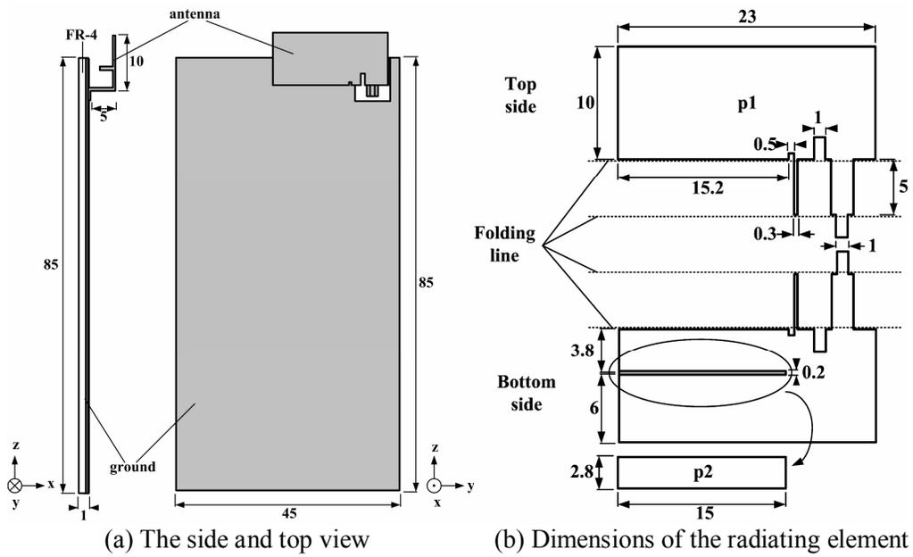
Fig. 1. Configuration of the proposed antenna for Bluetooth/WLAN applications.
