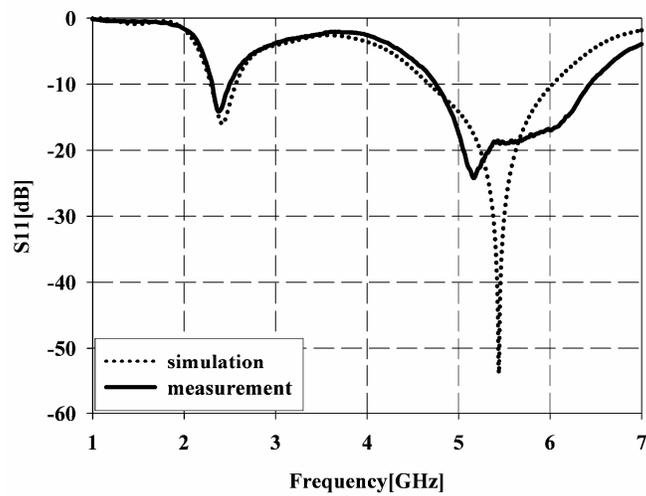
Fig. 2. Simulated and measured return loss for proposed antenna.
