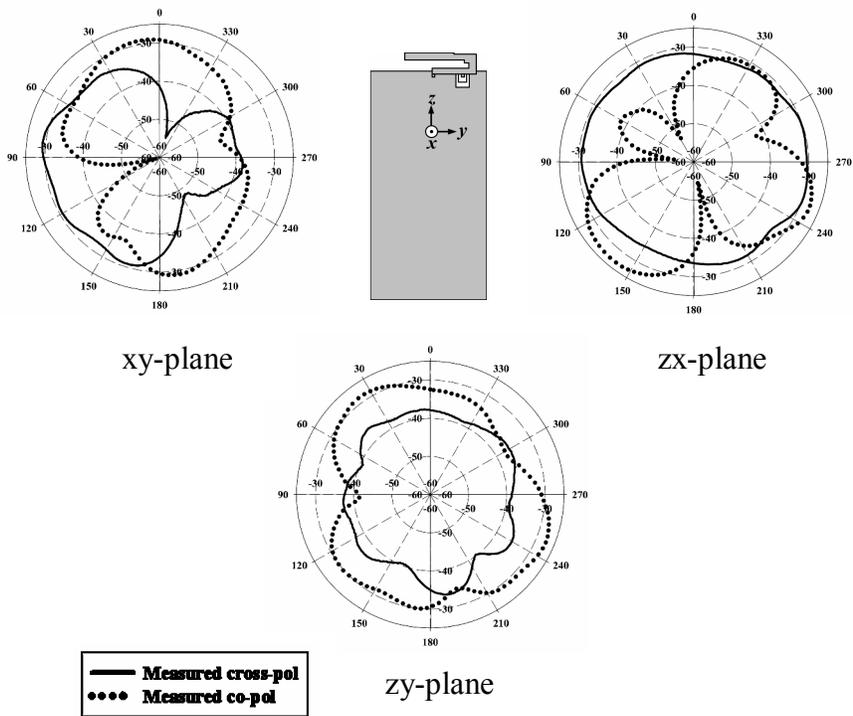
Fig. 3. Measured radiation patterns at 2.4 GHz
