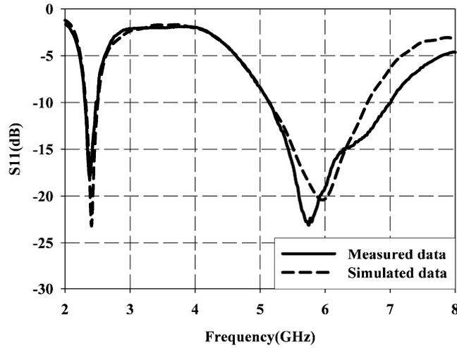
Fig. 2. The measured and simulated return losses of the proposed antenna
