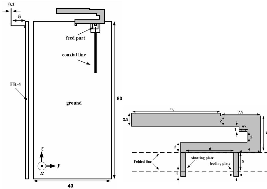
(a) The side and top view                      (b) Detail dimensions of the antenna
