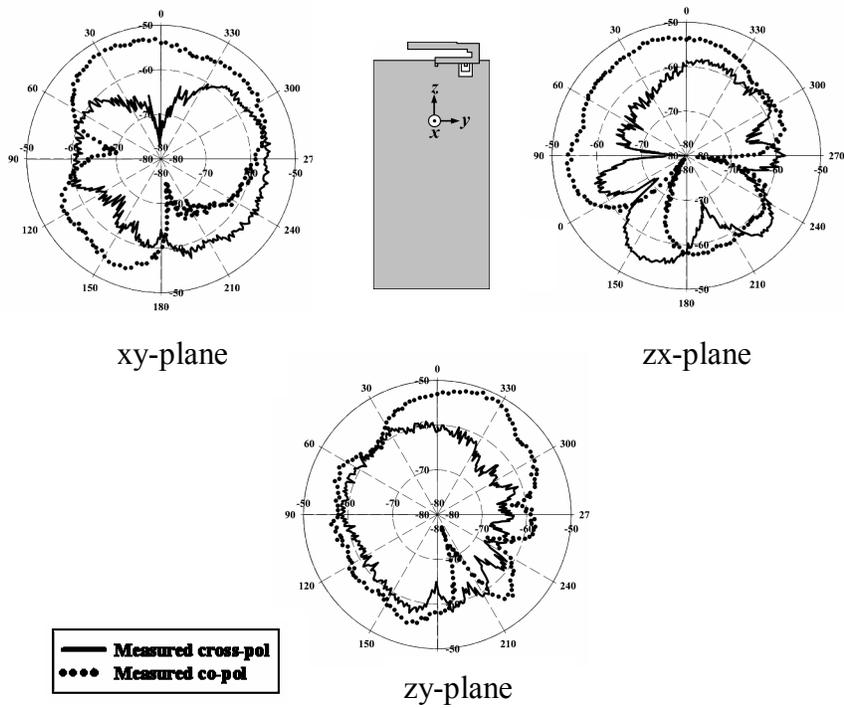
Fig. 4. Measured radiation patterns at 5.725 GHz
