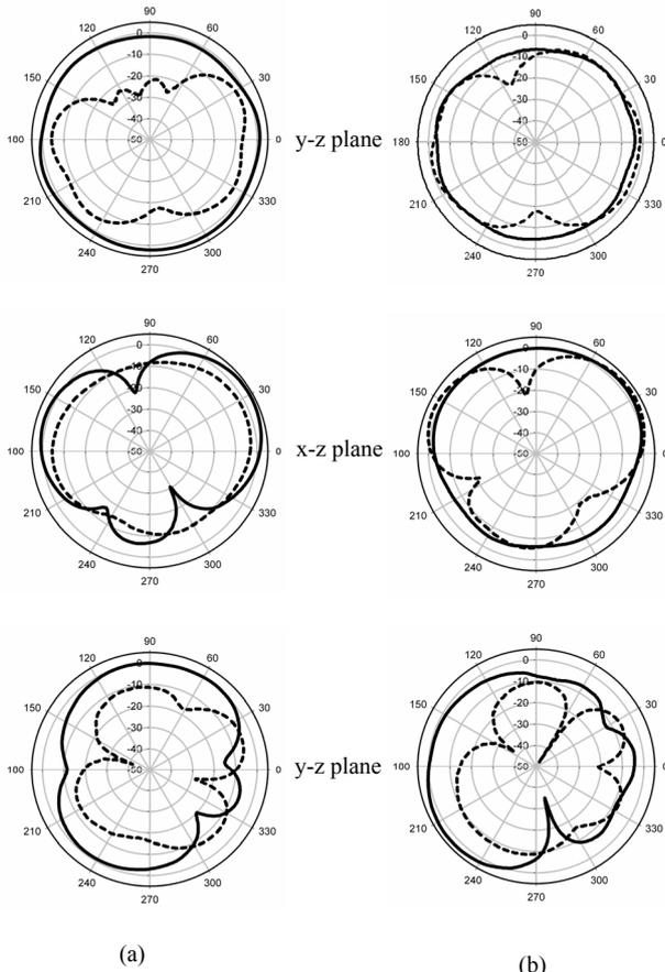
Fig. 4. Measured radiation patterns (a) 2.0 GHz (b) 2.35 GHz
