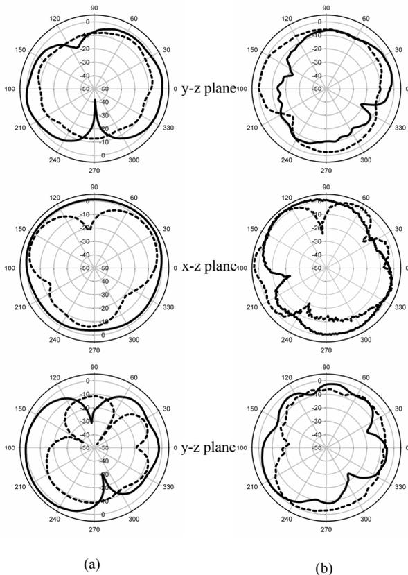
Fig. 5. Measured radiation patterns at (a) 2.42 GHz (b) 5.3 GHz
