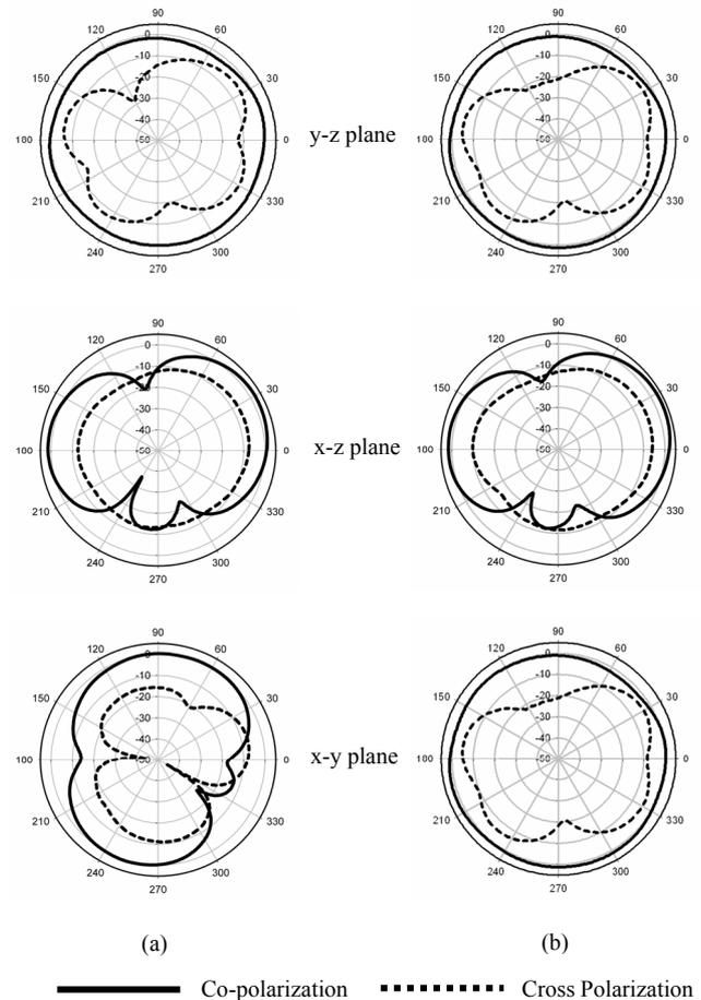
Fig. 3. Measured radiation patterns at (a) 1.71 GHz (b) 1.8 GHz
