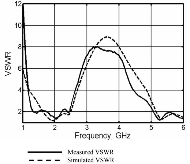
Fig. 2. Simulated and measured VSWR of the proposed antenna
