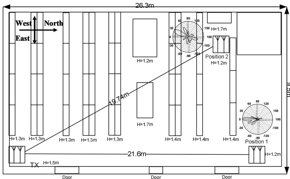
Fig. 1. 4X4 MIMO measurement environment
