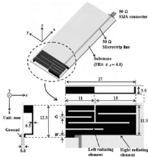
Fig.1. Configuration of the proposed internal antenna for PCS/IMT-2000/Bluetooth triple-band mobile phone.
