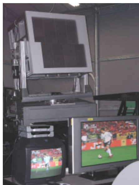
Fig 6. Satellite communication test of X-band APAA
