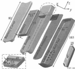
Fig. 7. Geometry of the handset case with battery
