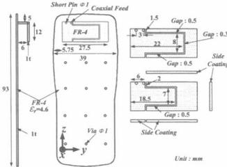
Fig. 5. Configuration of the modified antenna
