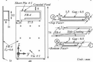
Fig 1. Configuration of the proposed antenna
