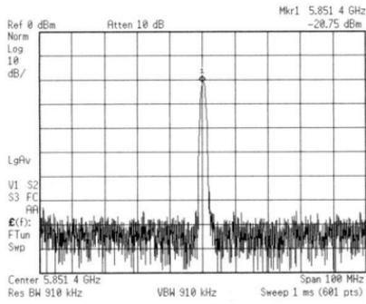
Fig. 3. Measured output power radiated from VCO antenna
