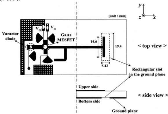
Fig. 1. Configuration of VCO antenna
