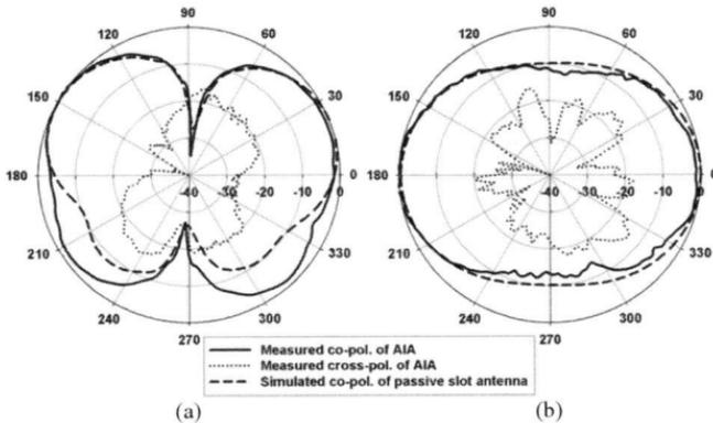
Fig. 5. Radiation patterns in (a) x-z plane and (b) y-z plane, at 5.8 GHz
