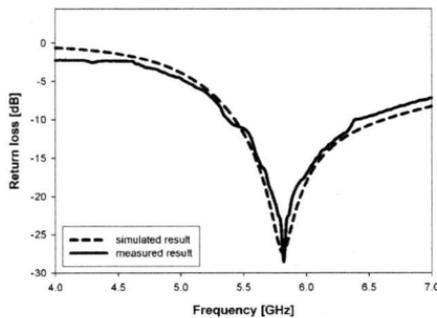
Fig. 2. Measured and simulated S-parameters for slot antenna
