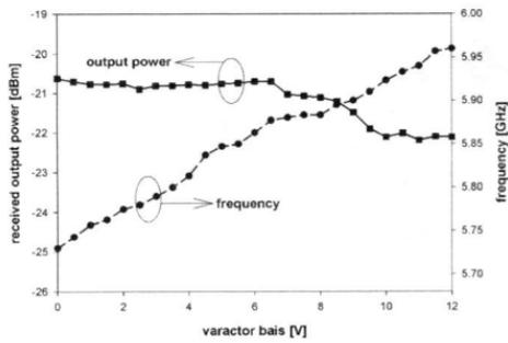
Fig. 4. Frequency and output power level in terms of control voltage
