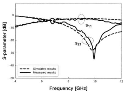
Fig. 2. Measured and simulated S-parameters for two-port slot antenna
