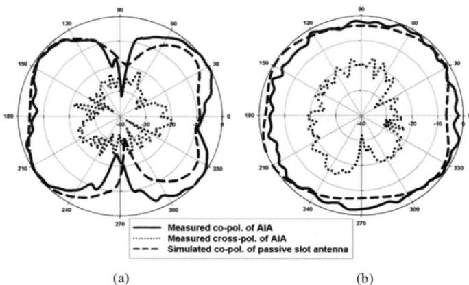
Fig. 4. Radiation patterns in (a) x-z plane and (b) y-z plane, at 10.05 GHz
