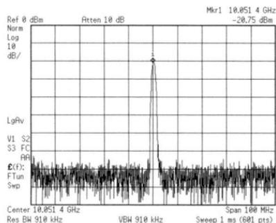
Fig. 3. Measured output power radiated from feedback antenna oscillator
