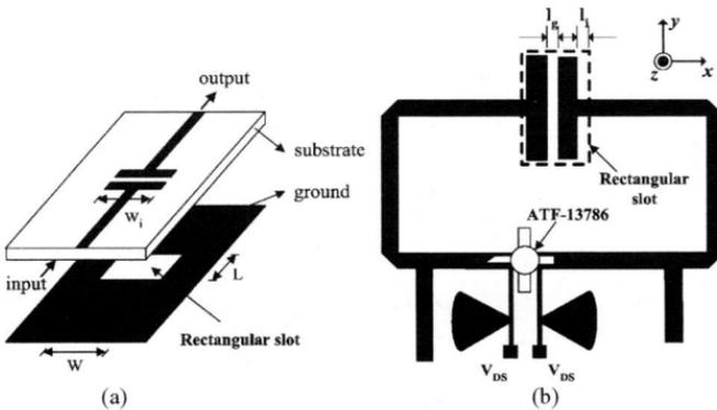
Fig. 1. (a) Two-port T-shaped microstrip-line-fed slot antenna. (b) Geometry of feedback antenna oscillator
