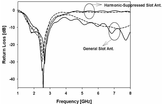
Figure 2. Simulated (dashed line) and measured (solid line) return losses for the proposed antenna
