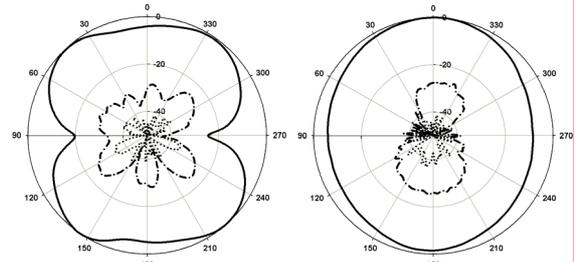
Figure 3. Measured co-polarization patterns of the proposed antenna (solid line : 2500 MHz, dash-dot line : 5000 MHz, dot-dot line : 7500 MHz)
