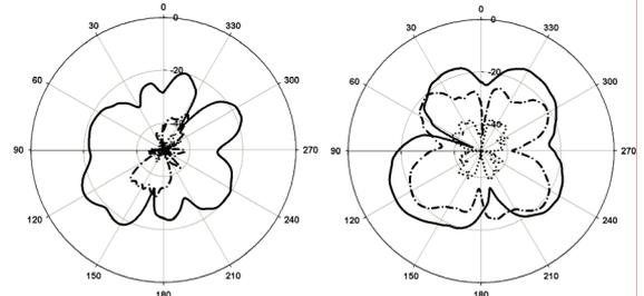
Figure 4. Measured cross-polarization patterns of the proposed antenna (solid line : 2500 MHz, dash-dot line : 5000 MHz, dot-dot line : 7500 MHz)
