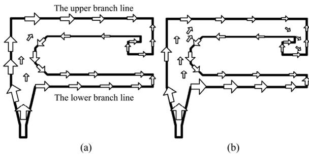
Fig. 5. Simulated current distributions on the antenna ⑥
