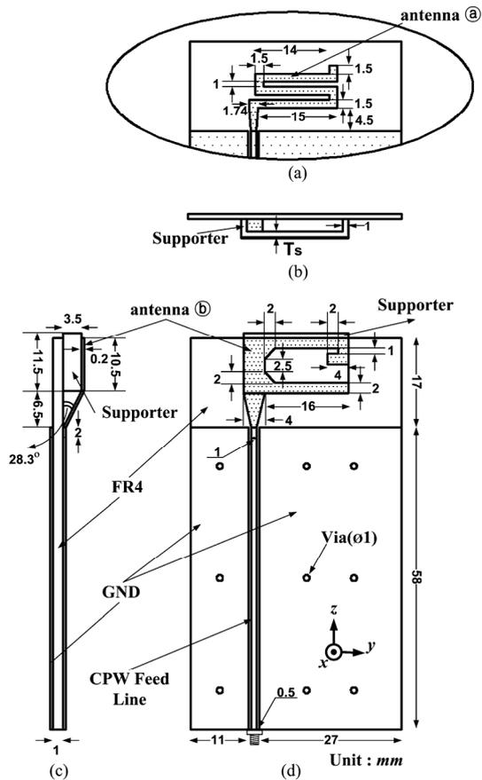
Fig. 1. Geometries and dimensions of the proposed wideband dual structure antenna.
