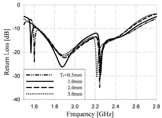
Fig. 3. Simulated return loss in terms of the different supporter's thicknesses ( $T_s$ ).
