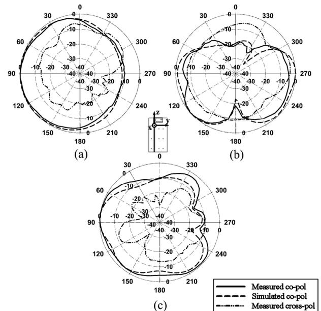
Fig. 7. Simulated and measured radiation patterns for the proposed antenna at 2.44 GHz.
