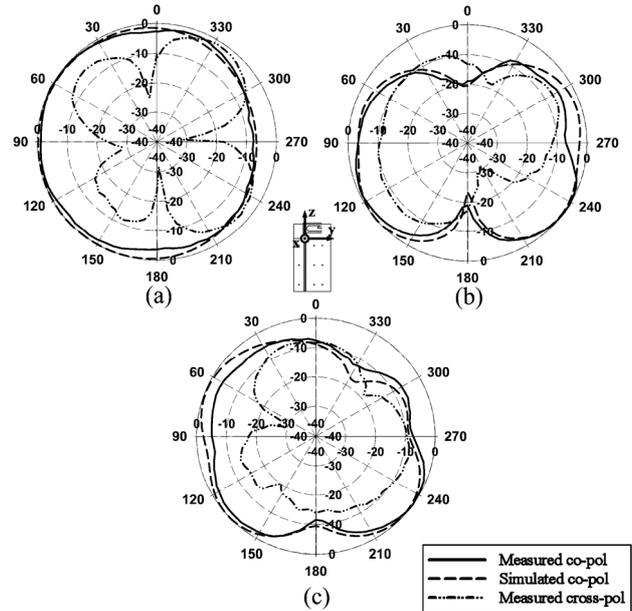
Fig. 6. Simulated and measured radiation patterns for the proposed antenna at 1.91 GHz.
