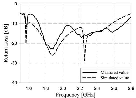
Fig. 4. Simulated and measured return losses for the proposed antenna ( $T_s = 1 \text{ mm}$ )
