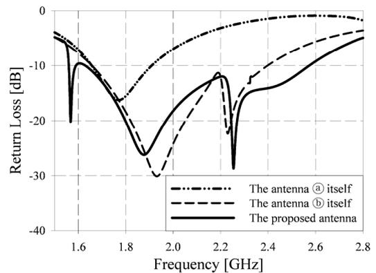
Fig. 2. Simulated return loss for each element.
