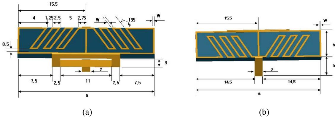
Fig. 1 The proposed antenna structure with Front view (a) and Back view (b)
