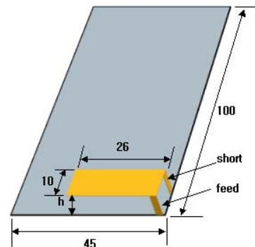
Fig. 3 PIFA mounted on chassis plane
