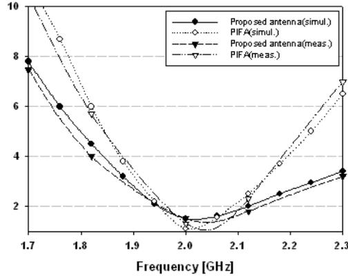
Fig. 4 Simulated and measured VSWR results between the proposed antenna and PIFA
