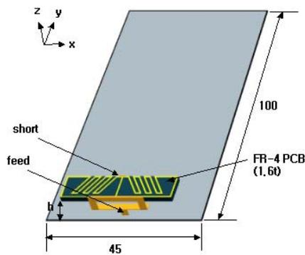
Fig. 2 Proposed antenna mounted on chassis plane
