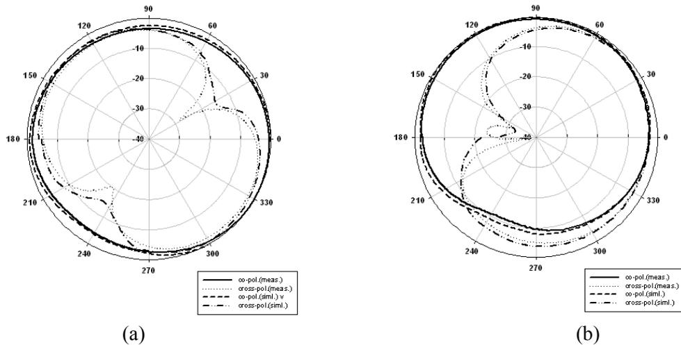
Fig. 5 Simulated and measured results of the radiation pattern at 2.0GHz for the proposed antenna (a) and PIFA (b)
