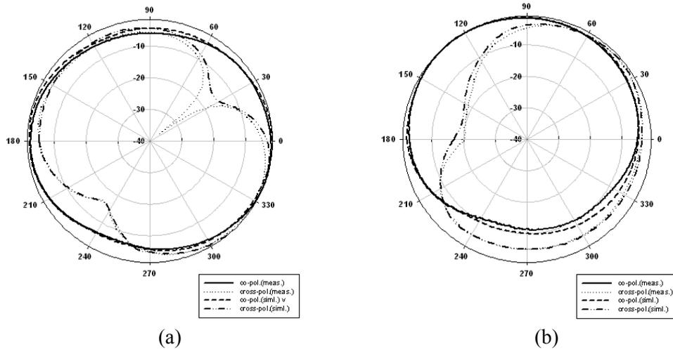
Fig. 6 Simulated and measured results of the radiation pattern at 2.05GHz for the proposed antenna (a) and PIFA (b)
