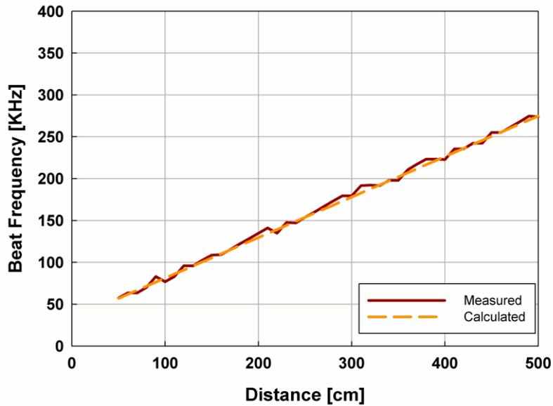
**Figure 3. Range measurement without frequency estimation**
