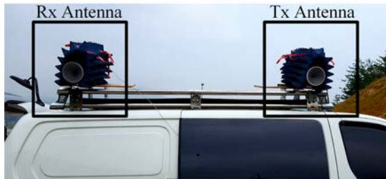
Fig. 8. Tx and Rx antenna configuration on a van.
