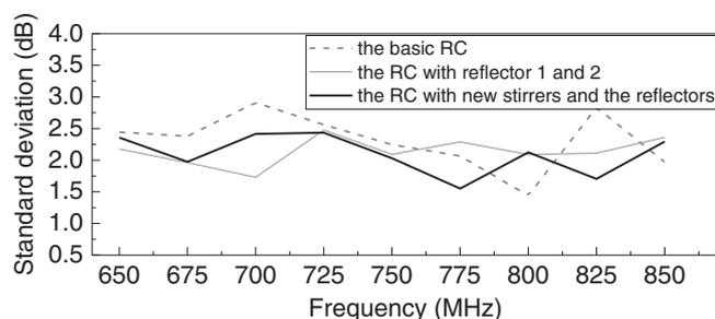
**FIGURE 3** Calculated standard deviations ( $\sigma_{xyz}$ ) for the RC with and without new mode stirrers and reflectors
