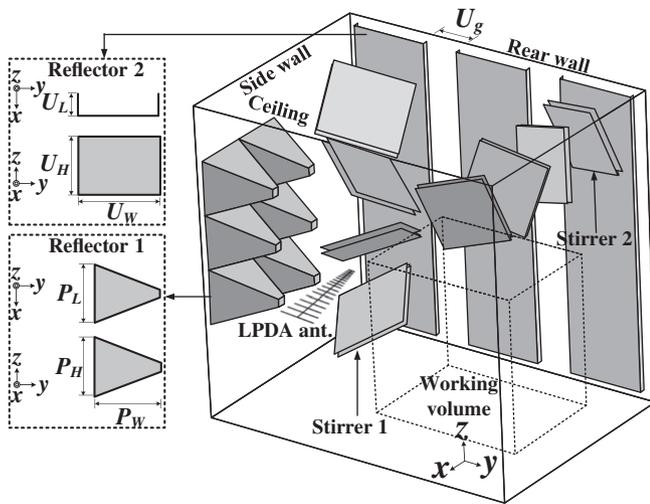
**FIGURE 1** The proposed RC structure with dual-type mode stirrers and 2 types of reflectors
