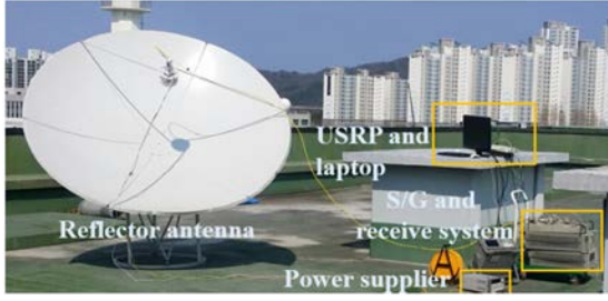
Fig. 6. Experimental setup for the GPS leakage detection in the outdoor environment.
