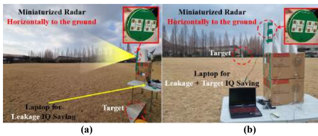
Fig. 12. Radar sensor experiment setup at KAIST Mun-ji Campus. (a) Experiment C setup. (b) Experiment C with targets.
