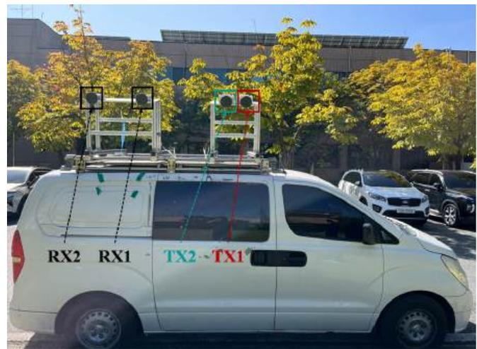
Fig. 7. A photo of SAR platform with the proposed SAR-GMTI system.
