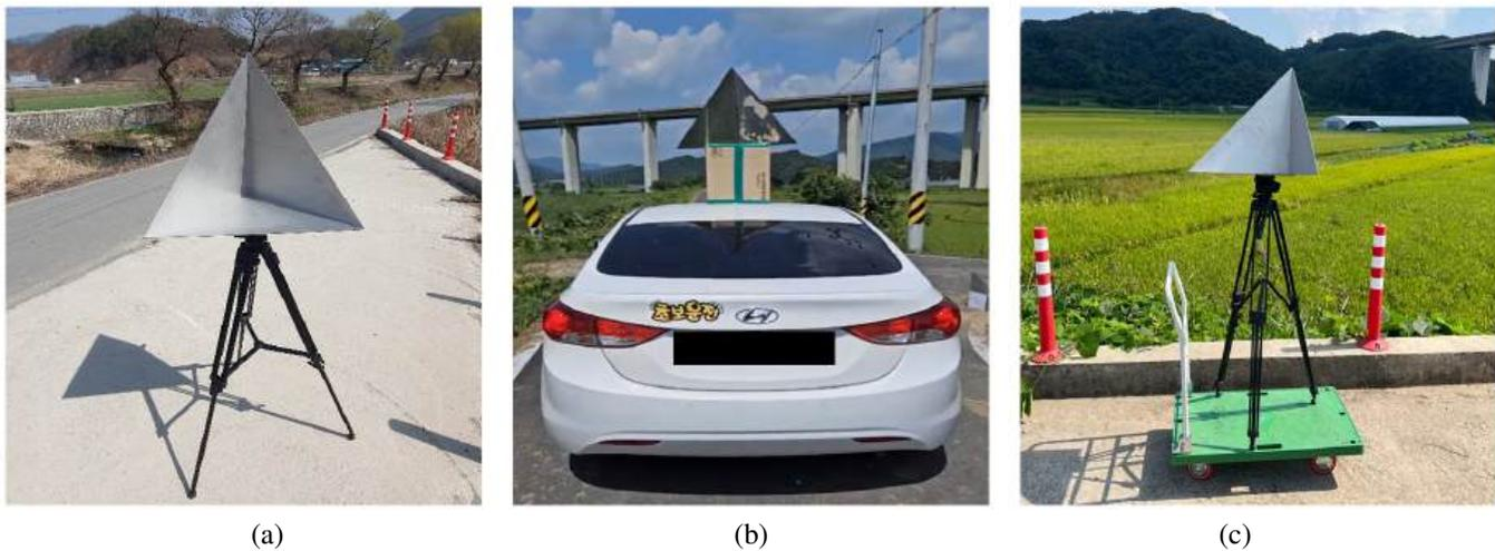
Fig. 9. Stationary and moving objects. (a) stationary object, (b) moving object #1 (automobile), (c) moving object #2 (trolley).
